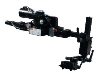
The Gullco remote controlled indexing system is typicaly used to automate a orbital overlay welding or surfacing applications. After each activation of the rotation limit switch the motorized arm will travel a preset distance, in a preset direction at a variabaly controlled speed (indexing) to produce the desired weld pattern. Variations on the process parameters are available to the operator through the easy to use programmable control.
